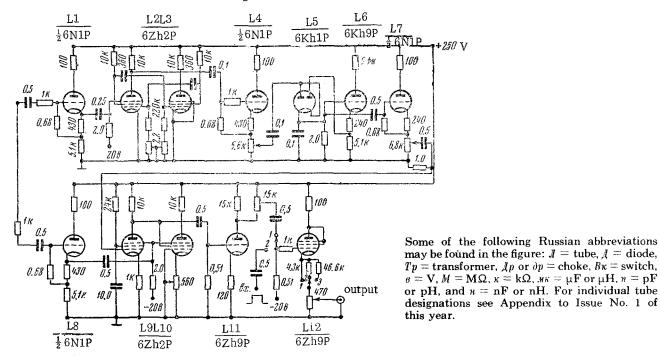
Fig. 2. Theoretical circuit of the apparatus.
